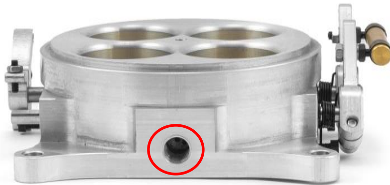
Figure 2: MAP sensor location Use barb fitting to attach MAP sensor
